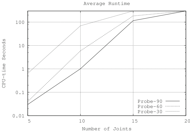
Fig. 7. Average CPU-time seconds needed by Probe to solve instances with j^* equal to 5, 10, 15, or 20, and g^* equal to 90, 60, and 30 deg, using the conditional model.
